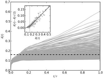
FIG. 2. Calculation of the bilayer melting threshold. Main figure: Time evolution of Lindemann parameters  $\delta_n(t)$  for all ice bilayers over a range of temperatures. Inset: Extraction of  $\delta_L$  from a piecewise linear fit of  $\delta_n(\tau)$  versus  $\delta_n(\tau) - \delta_n(\tau/2)$ . The fitted value of  $\delta_L$  is indicated with dashed lines.
